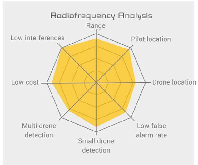
**Radiofrequency analysis** is the most balanced detection technology in order to:
